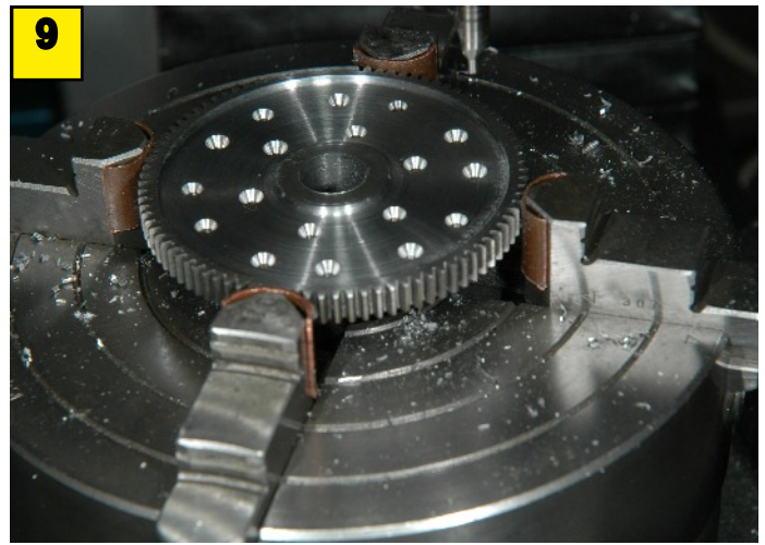
9 Template Removed Showing the Spot Drilling
