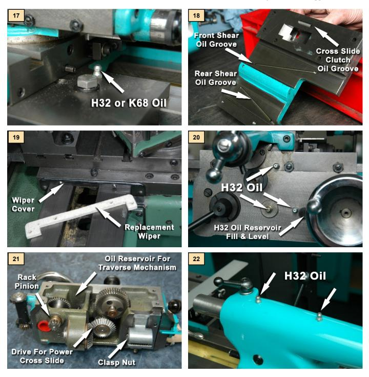
**Photo. 22** whilst the thrust bearing on the Super 7 is lubricated through the oil nipple in **Photo. 23** again with H32
