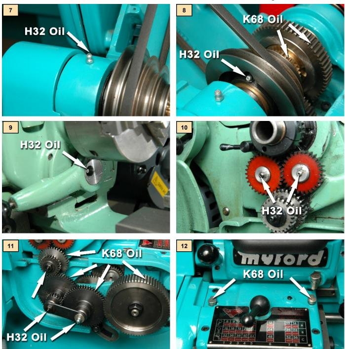
cient oil is required to eliminate the friction without splashing oil all over the surrounding areas. For lathes fitted with a Q.C. gearbox the gearbox requires lubrication entirely with K68 oil which is a gearbox oil.
