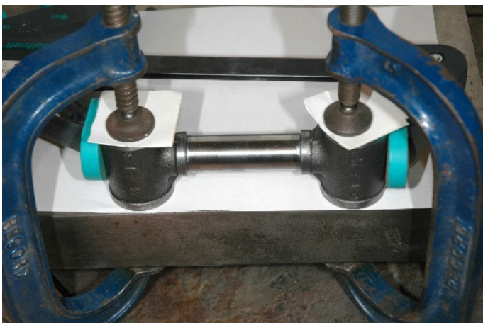
Photo. 8 Assembling with Epoxy Resin
