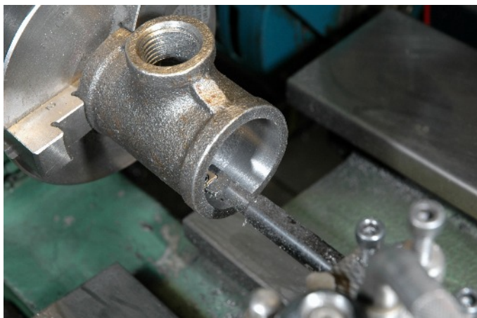
Photo. 2 Boring Out for the Pillar Sleeve
