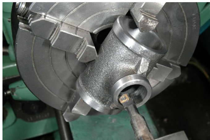
Photo. 3 Boring Out for the Cross Arm
