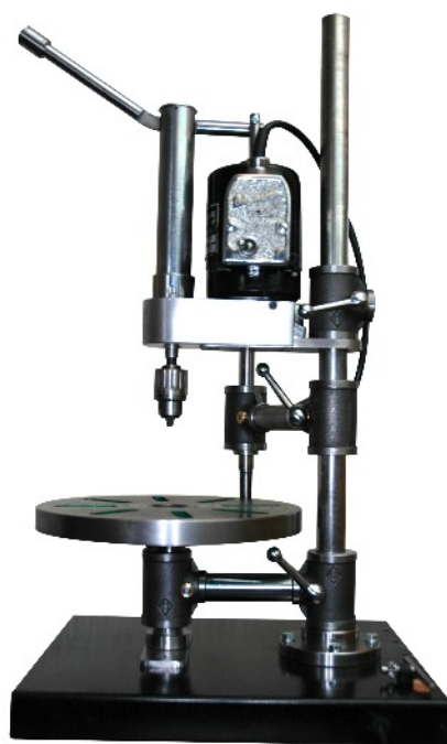
Photo.17 The Pillar Tool Used for Drilling.
