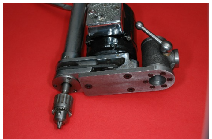
Photo. 15 Mounting the Drilling Head.
