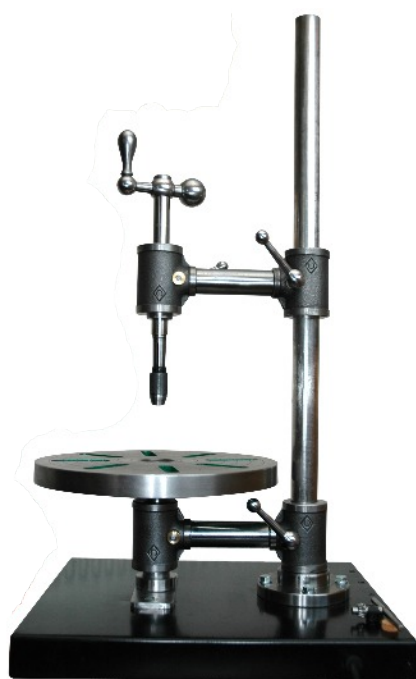
Photo.16 The Pillar Tool Used for Tapping .
