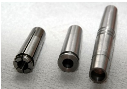
Photo. 12 Finished Collet showing the manufacturing Stages
