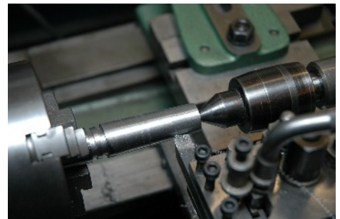
Photo. 9 Turning The Number Two Morse Taper
