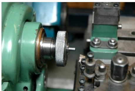
Photo. 2 The Short Overhang of Myford Collets
