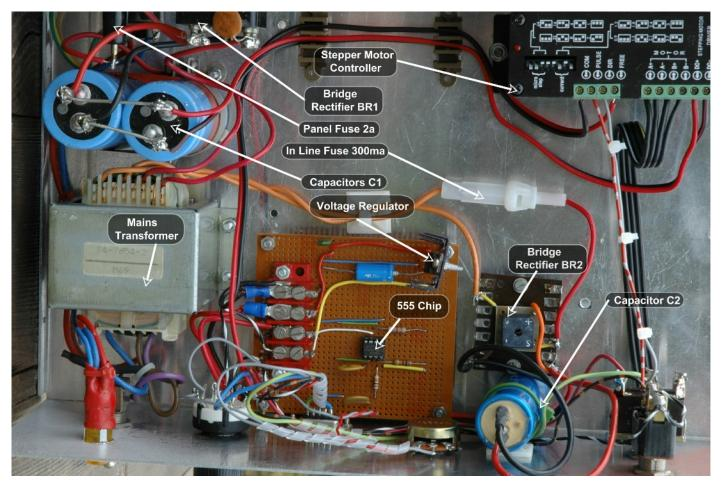
voltages which are not smooth. The Electrolytic capacitors C1 & C2 smooth these DC supplies to give two smooth, constant DC outputs.
