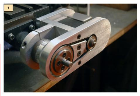
chine. I did however design the drive so that it can be rotated about the leadscrew and used in any position, as I believe is the case with the factory supplied drive. To the left of the graduated dial is a machined recess 30mm Dia. and 15mm wide to which Wabeco attach their motor drives and I decided that my fixture would clamp to and swivel about this point.
