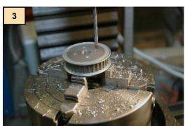
was then drilled to 9.5mm and finally bored out to 10.1mm. The material was fairly hard but machined well. I held the pulley by the fixing flange (as in Photos 3 & 4) rather than risk damage to the aluminium belt flanges. You will remember to remove the grub screws before drilling and boring won't you?
