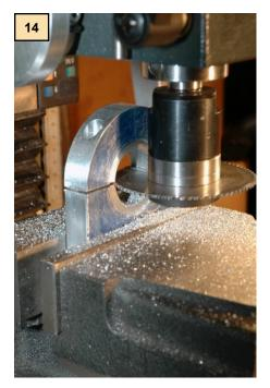
nor did I drill the holes in part C for the fixing set-screws to attach to part D. Having clamped part A to the Wabeco, I assembled the whole thing "loose" and made sure that the required position for the fixing holes and counterbores in parts D & C were actually where the drawing stated once the belt was tight and running truly in the
