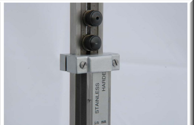
Photo. 13 The Readout Bar Clamped In Place
