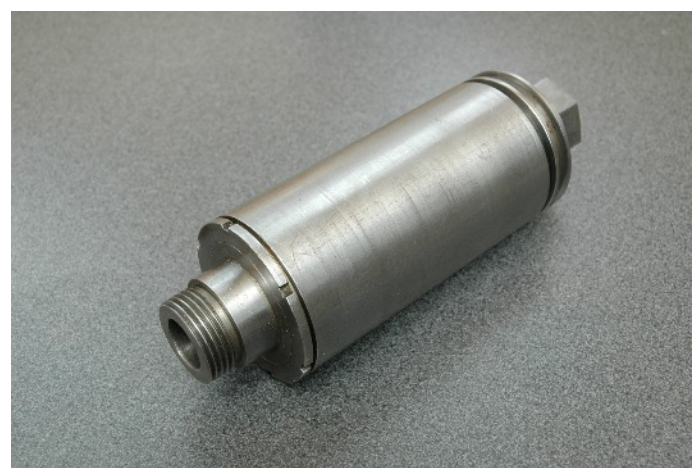
Photo.5 Finished spindle ready for use
