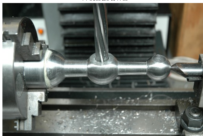
Photo. 9 Milling the Flats and Reaming the Holes
