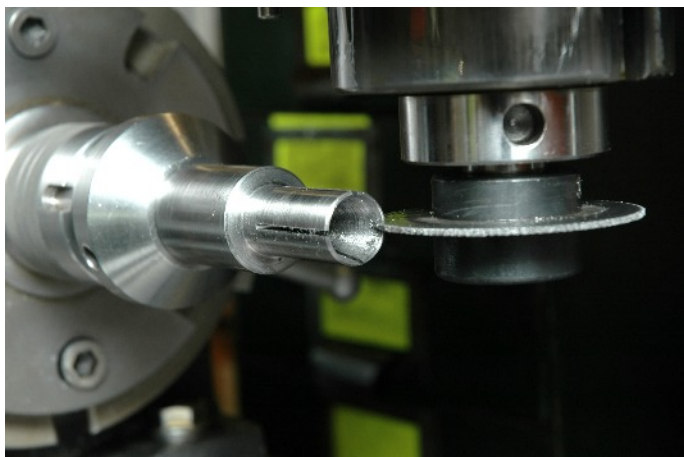
Photo. 12 Slitting the Mandrel Extension
