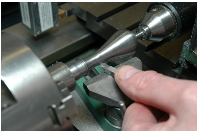
Photo.10 Using a Hand Turning Rest
